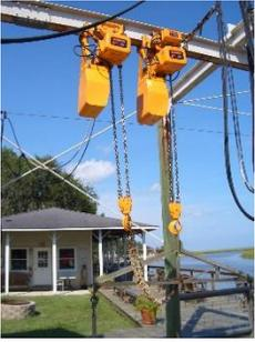
The hoists are working well, thanks to some rework on the control wiring by Steve Ellis, but occasionally someone will forget to put them back under cover when done. Once water gets into the case, they soon develop electrical problems.
